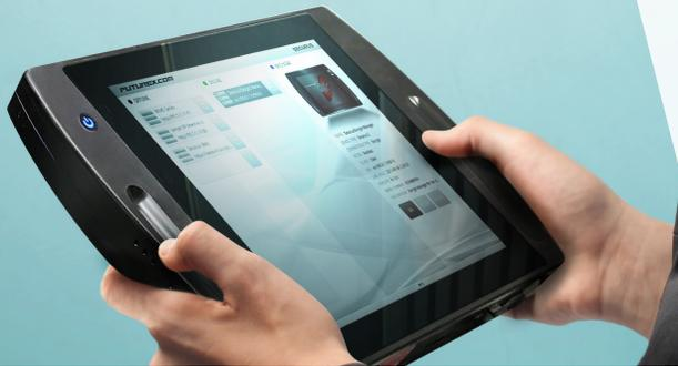
*The Excrypt Touch is unique in that it's a portable tablet that incorporates a FIPS 140-2 Level 3 compliant HSM—the only one of its kind on the market. This allows users to conduct remote device management procedures with comfort and convenience. As a hand-held device, it can be used without a monitor, mouse, or keyboard, and can be passed between key officers without being confined to a rack.*
